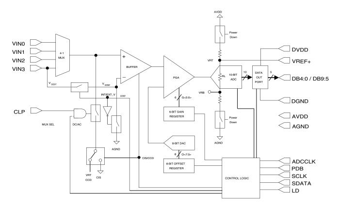
Figure 2. Functional Block Diagram of XRD9829
